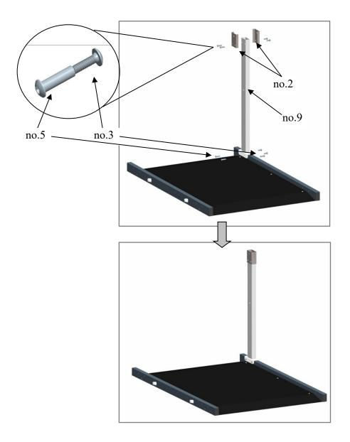
Step 2. Assemble pole on platform, as per Step 1.
