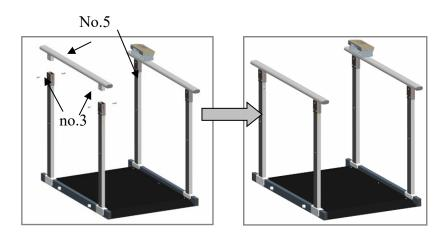
Step 6. For M-652, assemble cross bar (SS-8444) with two screws (M8-1.25P\*45).
