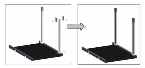
Step 3. Attach no.1 (handrail bar) to poles, using no.3 (socket screw) and no.5 (screw nut).
