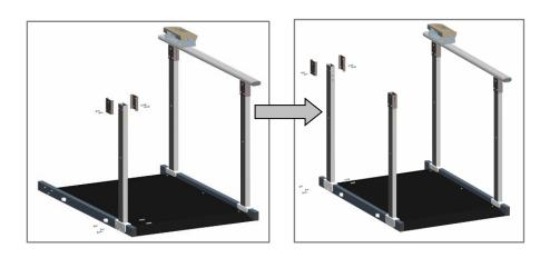
Step 5. With handrails assembled, attach no.13 (bracket for indicator) using no.6 (screw)
