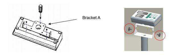
1) Place Bracket A on the back of the indicator with three screws as shown in the image above.
