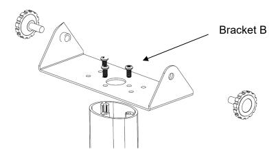
2) Place Bracket B on the top of the column using three screws (item 8).
